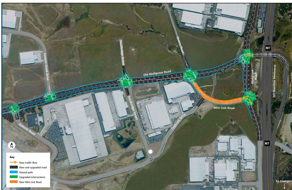
Figure 6: Old Wallgrove Road Completed Upgrades
